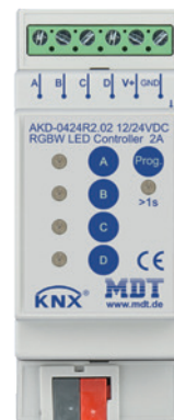
The MDT AKD LED Controller 4-channel (AKD-0424R2.02) dims 12/24V CV LEDs. The LEDs can be controlled as four individual channels, as Tunable White, RGB and RGBW.
