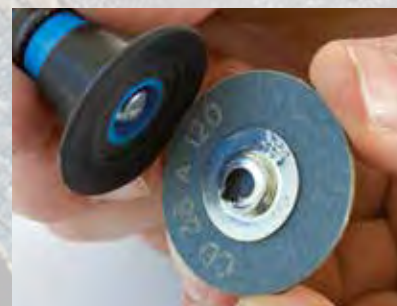
304 Abrasive discs with rapid clamping fastener COMBIDISC®
