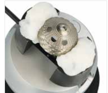
Mould jaws made of modelling granulate
