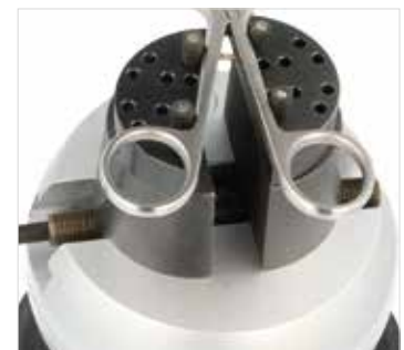
Mounting via retaining pins
