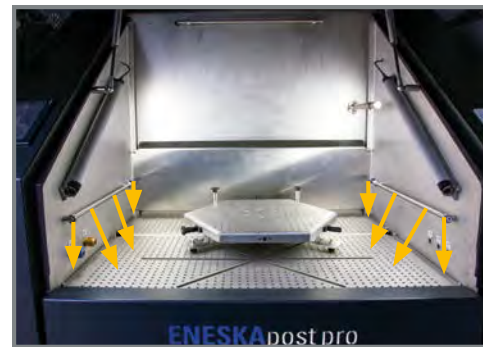
After the processing, the system cannot be opened until a special automatic cleaning process has finished. This stirs up and extracts the residual dust from the corners of the chamber.
