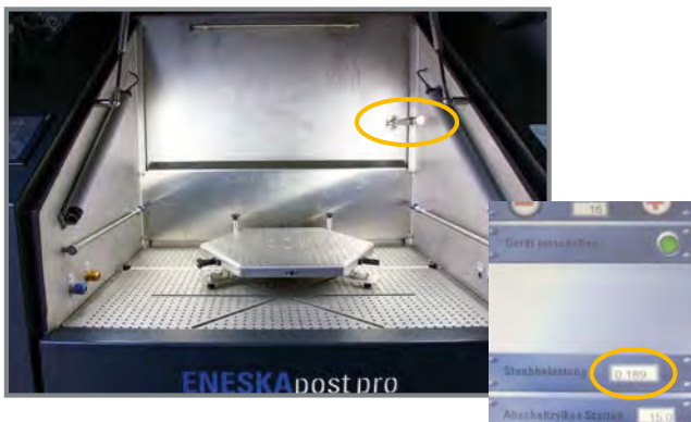
The system can be equipped with the special FSX automatic fine dust measurement. The dust load in the working chamber is continuously measured and shown on the display.
