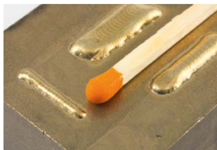
Welding seam build-up - bronze material
