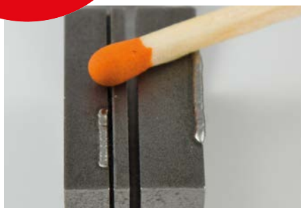
Welding seam build-up - steel material
