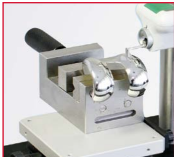
Measurement of a knee joint with drive unit MarSurf RD 18 and skidded probe system PHTR-100
